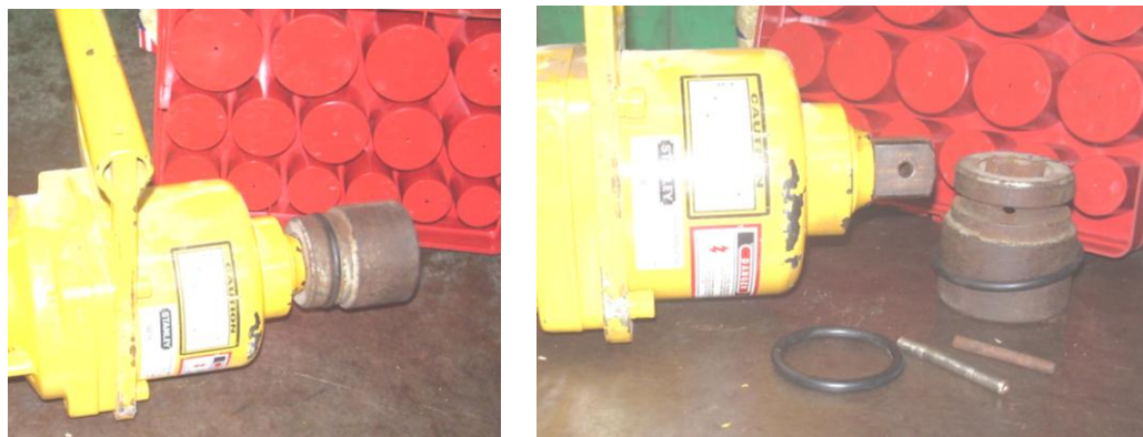
Showing correct size and length of retaining pin to secure the socket
