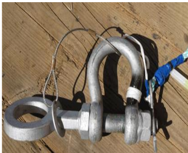
Example of shackle with welded modification performed by supplier
