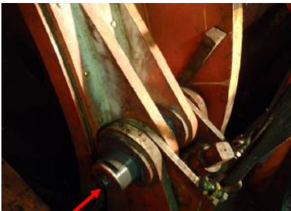
Installation of brake pin using hydraulic jack (red arrow)
