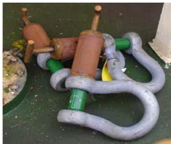
Example of shackle with welded modification performed at worksite
