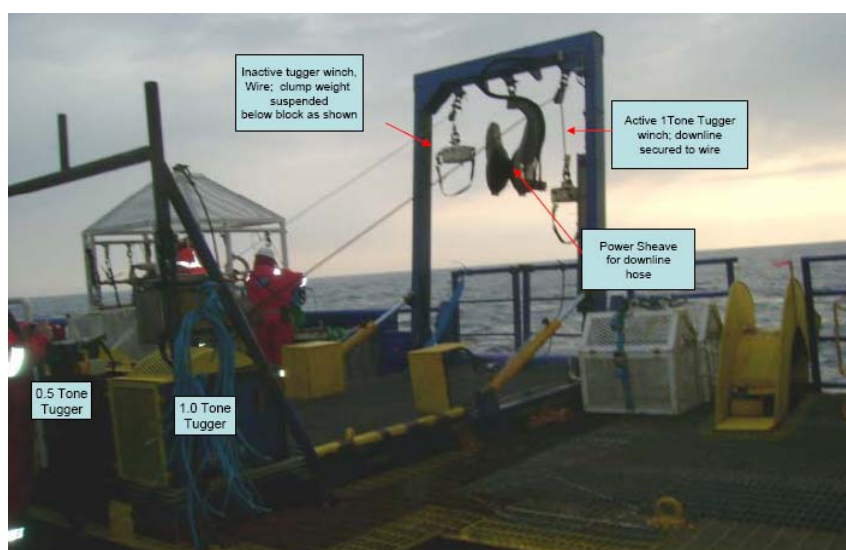
A-frame with tigger winch, snatch block and powered sheave arrangement
