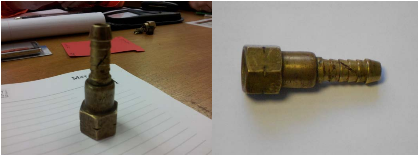
Damaged acetylene fitting
