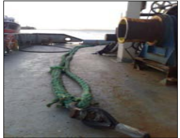
Figure 5 - Mooring rope similar to that used in the operation
