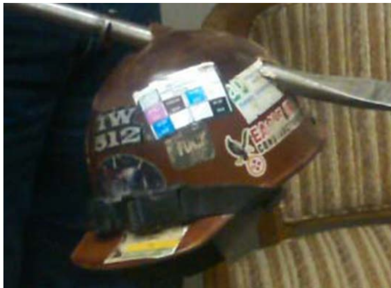
Figure 1 - hard hat destroyed by falling sleeve bar
