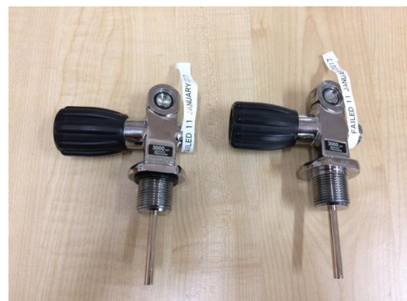
Example of New Pillar Valves that FAILED
