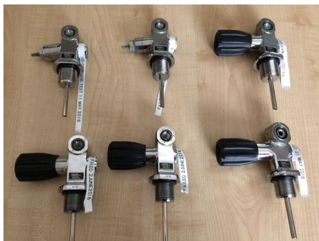
Six In-Service Pillar Valves that FAILED
