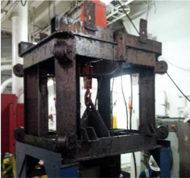
Figure: Multibeam carriage before deployment to moonpool
