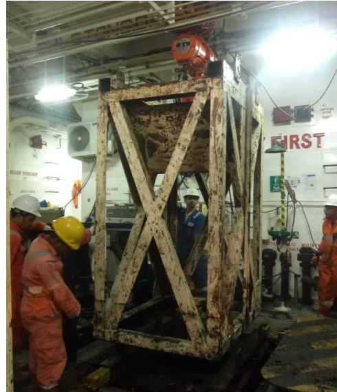
Figure: Frame before deployment to moonpool, attached to multibeam carriage underneath
