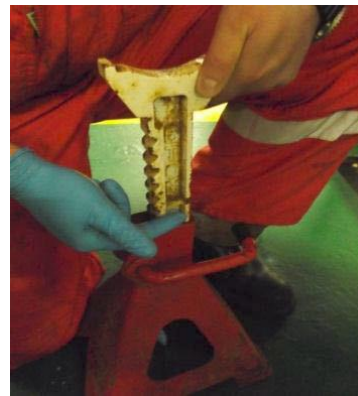
Figure: Illustration of where finger was pinched during adjustment of the axle stand
