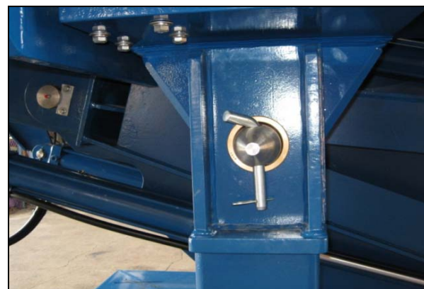
Example of future locking pin design with retaining pin
