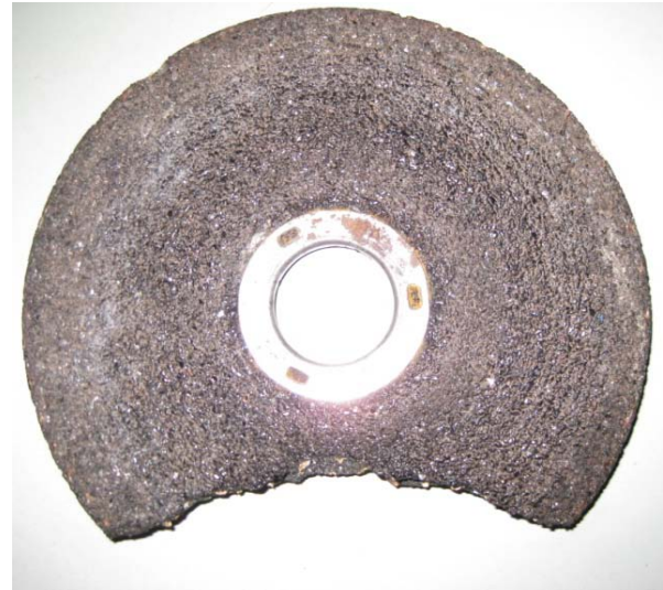
Broken grinding disk after inappropriate use
