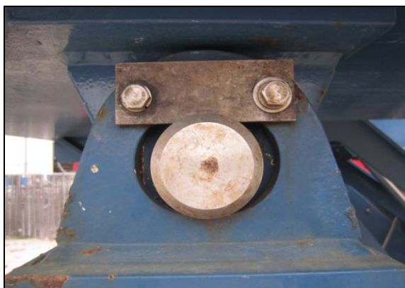
Example of other lift post pin locking configuration
