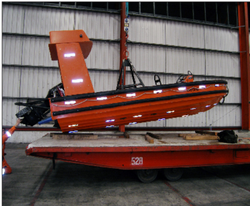
Weighing of the rescue boat
