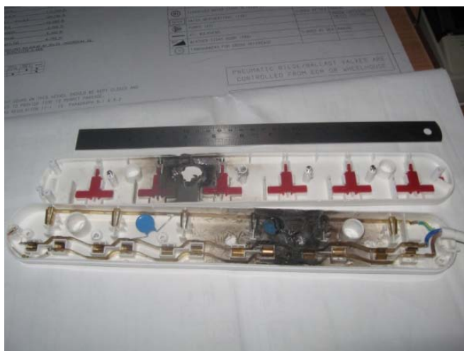
The inside of the 6 way socket extension, showing the damage caused inside the unit
