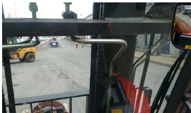
Showing drivers view from inside cab – blind spot
