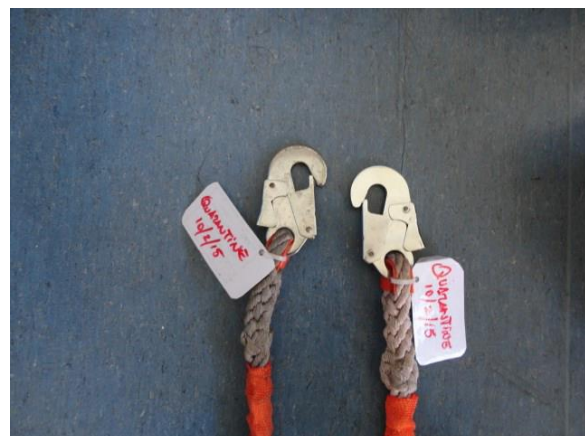
Figure: showing hooks with faulty safety clips
