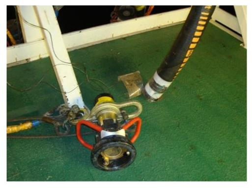
Figure - Mud hose and connector following incident
