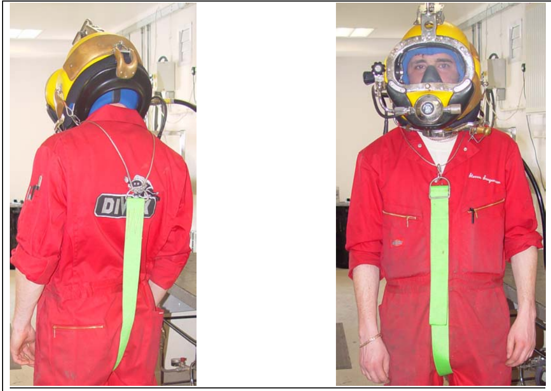
figure 2 showing front & rear view with shoulder wires located in helmet side strop assy hooks and jock strap adjusted to be comfortable.
