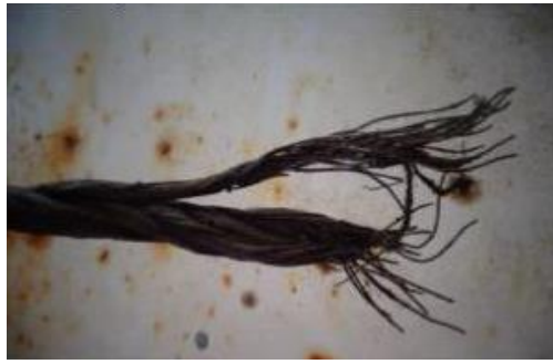
Break following ineffective maintenance of gangway wire
