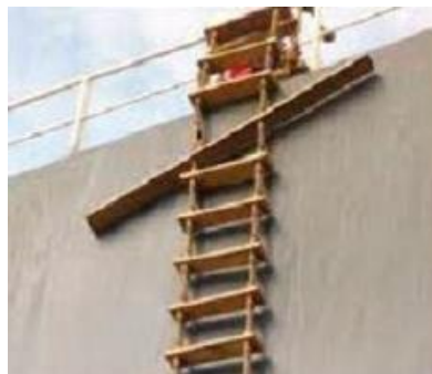
Missing chock and steps unsafe for boarding
