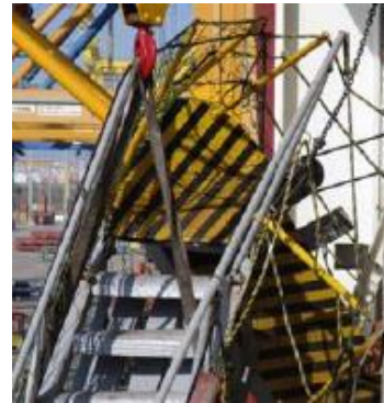
Wrong operation of gangway
