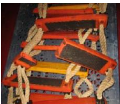
Broken step on a pilot ladder
