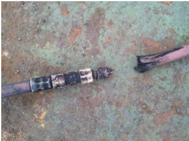
Figure: Showing damaged hoses after fire
