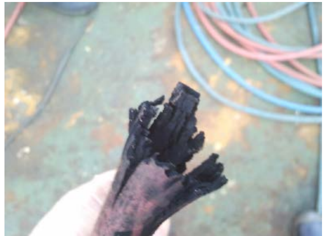
Figure: Showing damaged hoses after fire
