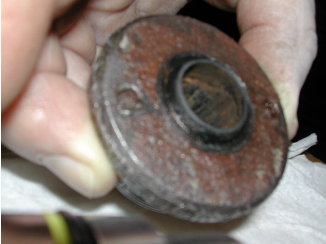
Picture 2. The end piece is corroded, also on the inside.
