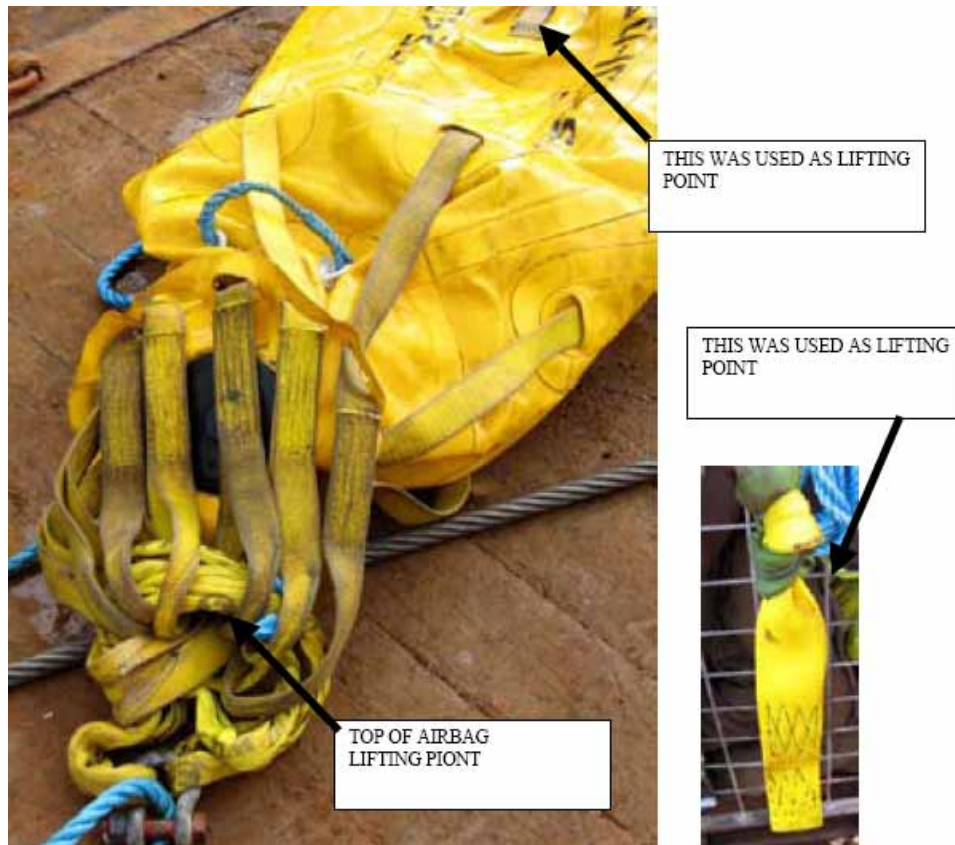
Lifting bag similar to that involved in incident
