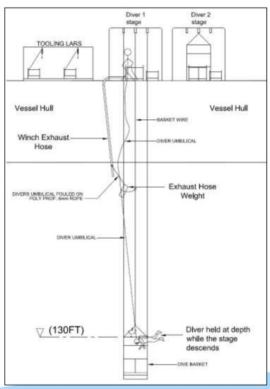
suspended exhaust hose and weight to "wander" more than usual. This in turn led to the entanglement of the weight with the carabiner:
