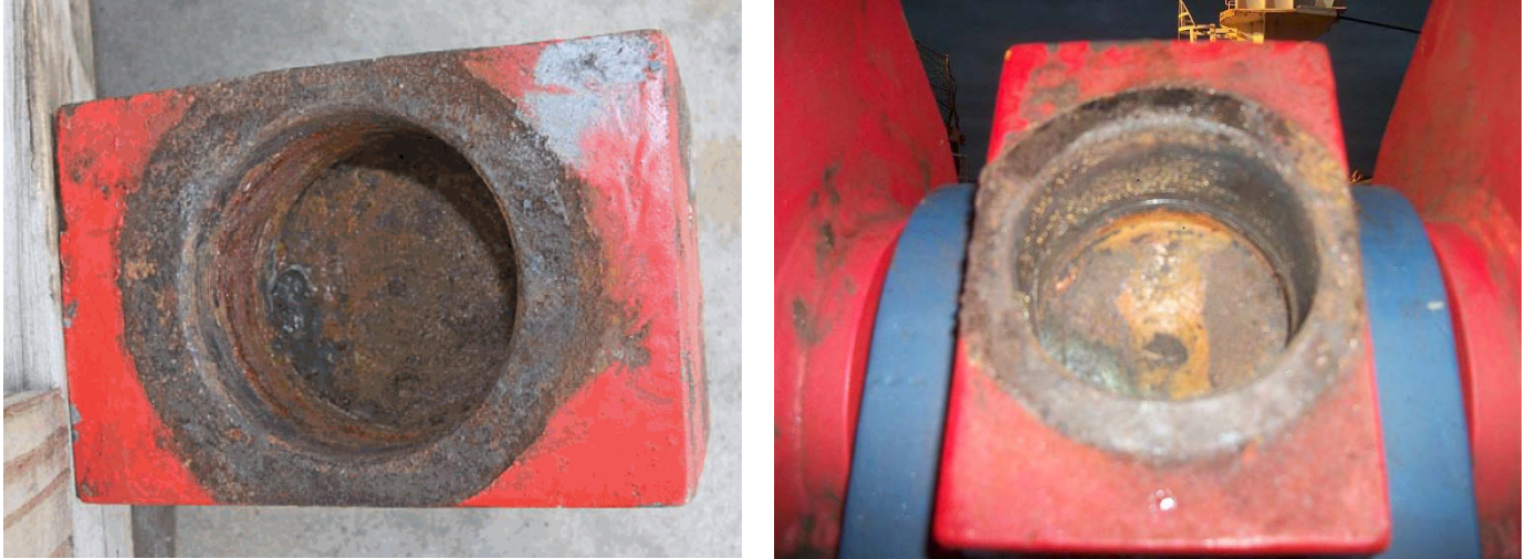
Clevis pictured after failures
