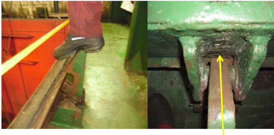
Spring-loaded latch operated by foot
