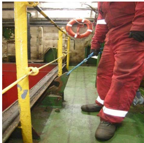
Showing rope tail in use (making manual handling unnecessary)
