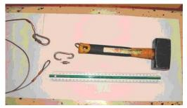
to a walkway below, which at the time of incident was completely sealed off. The hammer, safety wire and two double sealed spring hooks were all tools dedicated and solely used for work in height.
